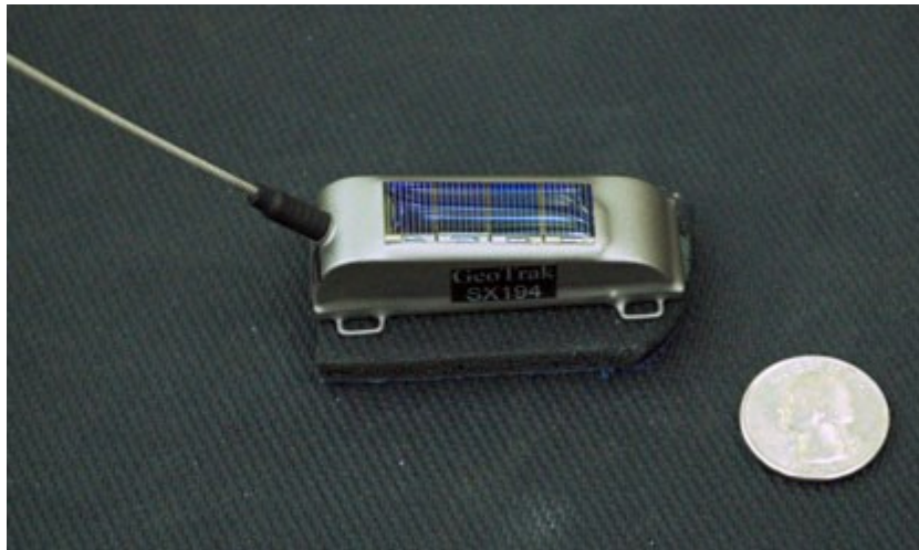
Satellite transmitter used to track select falcons.
